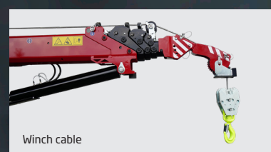
Adjustable section with manual jib extension
